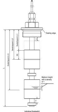
Individual floatswitch Example made from PVC with a connection cable
